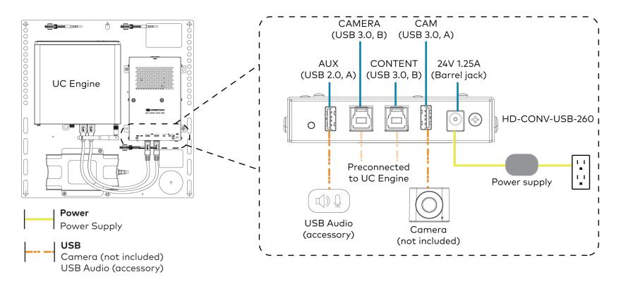
3. Connect power, the content ingest device (HD-CONV-USB-260), and LAN to the top of the UC Presentation Transmitter.
